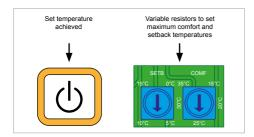
Temperature control for Setback period, For this mode, the switches are set as shown below.
