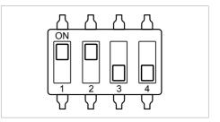
In timer mode, switch 3 or 4 must be in the 'ON' position. This mode allows for 3 different settings which will alter the time period for each segment.
